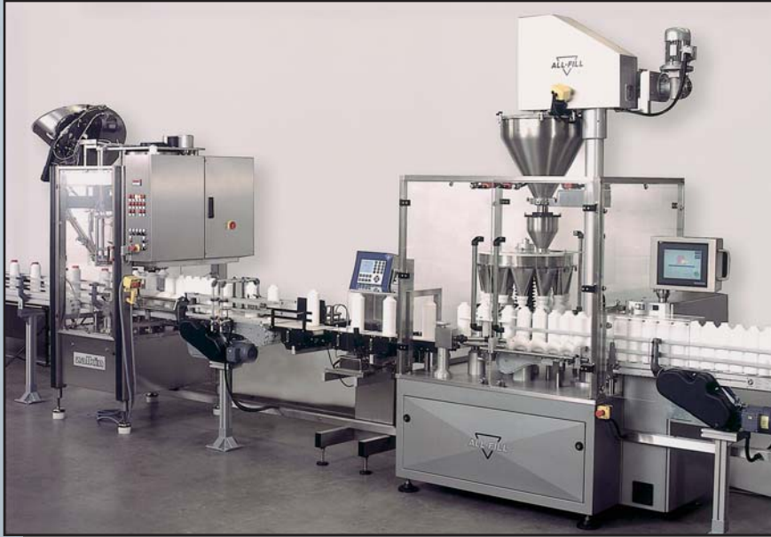
A 120 per minute line for garden products with checkweigher feedback and screw capping.
