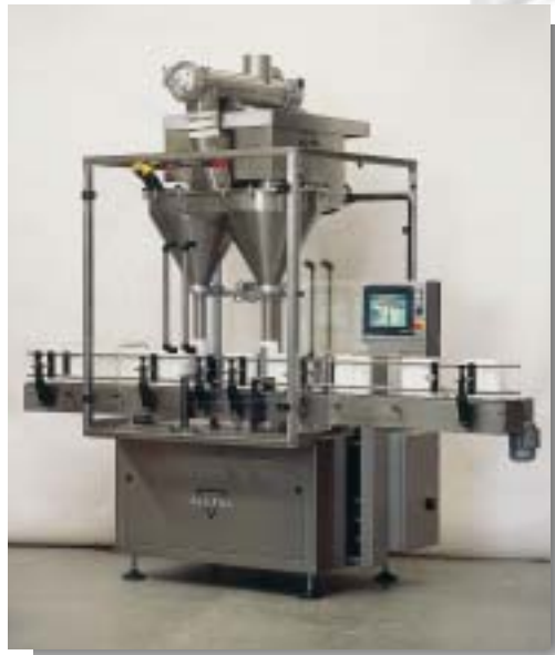
Series 200 twin head filler with compressive bottom-up filling of health food powders, and single horizontal auger feeding.
