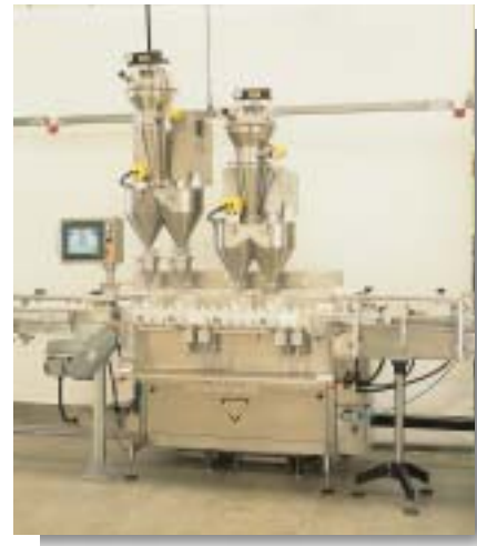
Special 4 head filler for dry suspension antibiotics with balcony configuration and wormscroll bottle handling.
