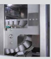
STERILINE linear washing machines **VW** series are designed to process vials up to 1.000ml with a capacity range up to **24.000 pcs/h**. Finishes range from mill finished to mirror polished. All welded points are argon atmosphere treated and then mechanically polished and passivated. The valves are high purity diaphragm type and pneumatically actuated; the pipe fittings are tri-clamp type and all piping is fully drainable.
