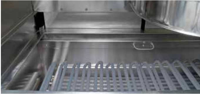
COOLING CHAMBER HEATING ELEMENTS
