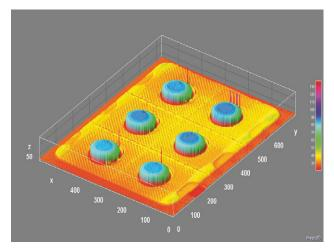
3D evaluation of a sealed blister for the recognition of sealing area and pockets.
