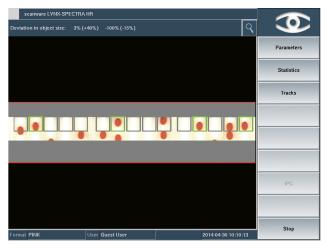
Evaluation of soft gel bulk. Due to optical varieties, the separation of the products is crucial.
