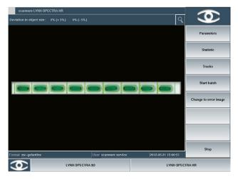
Evaluation on a large scale bulk inspection machine. The products are lined up by plastic skewers and presented to the camera. Separation of the product is not necessary.
