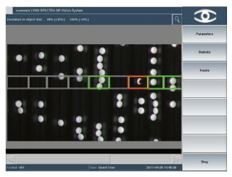
Evaluation on a vibratory feeder. The separating of the products that are randomly distributed on the lanes is undertaken by the software. Afterwards, product inspection takes place.
