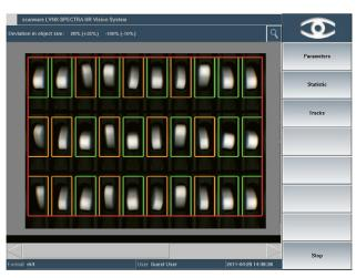
Evaluation on a slat counter. The upright products are inspected and signals processed. The above screenshot shows cross-contarmination with smaller objects.
