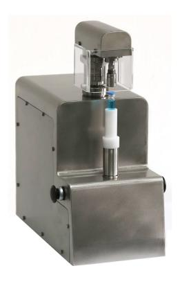
The operator places the aluminum crimp cap manually onto the vial and places the vial in the container centering device. Upon activation of the two-hand control the vial is lifted towards the plunger. The plunger rotates the vial while the crimping disc swivels in place and asserts pressure onto the crimp cap. The disc gently folds the aluminum cap around the neck of the vial and secures the crimp cap to the container tight and securely.
